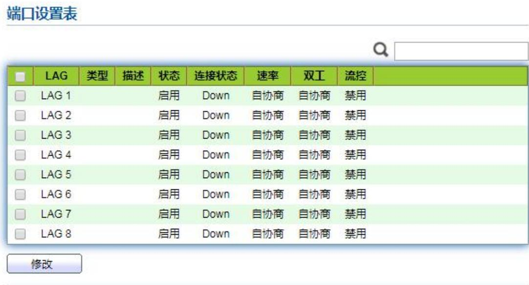
The screenshot shows a table titled '端口设置表' (Port Settings Table) with 8 rows, each representing a LAG. The columns are: LAG, 类型 (Type), 描述 (Description), 状态 (Status), 连接状态 (Link Status), 速率 (Rate), 双工 (Duplex), and 流控 (Flow Control). All LAGs are listed as '启用' (Enabled) with 'Down' link status and '自协商' (Auto-negotiation) for all other parameters. A '修改' (Modify) button is located at the bottom left of the table.
